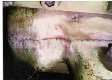
2600 TON PRESS CROSS HEAD MARKING AFTER COLOR CHECK
